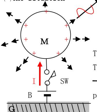
**G** is earth of voltage=0. **B** is battery connecting to monopole antenna **M** through switch **SW**. **M** is a sphere of conducting surface. Making **SW** on causes **M** equi-voltage of **B** by flowing charge(current) on **M**.
