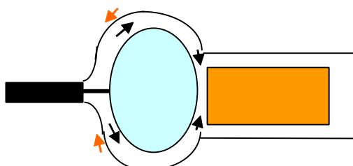
A high frequency current dislike abrupt curvature surface.
