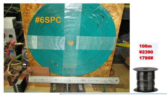
Center hole D=2cm( $\pm 5$  coin) L2 diameter 2R=27cm(54t) L1diameter 2R=29cm(4t)  $\Delta R=(27-2)/2x54=0.23$ cm/t \*winding method $\rightarrow$ Part I 3(3)
