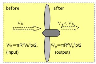
If we could  $V_a=0(\eta = 1)$ , then maximum efficiency could be accomplished. However normal wind turbine could not,but  $\eta < 40\%$ . (c)Below is modified version by author. Cone acts as **pressure amplifier** with high efficiency(however,this is not assured by experiment).
